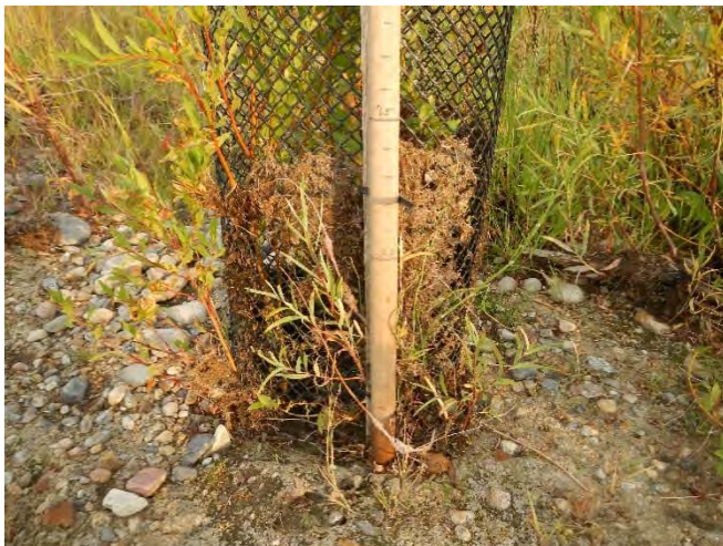
Photos 1-3. High water indicators from 2017 that indicate approximately bankfull conditions in Phase 5-6 (only localized floodplain overflow).
